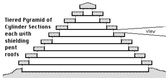
A less pretentious example of sky-scraping is given in the end-view cross-section sketch below, where a number of horizontally placed cylindrical pressure hulls are stacked. The advantage is in longer rectangular floor space.
