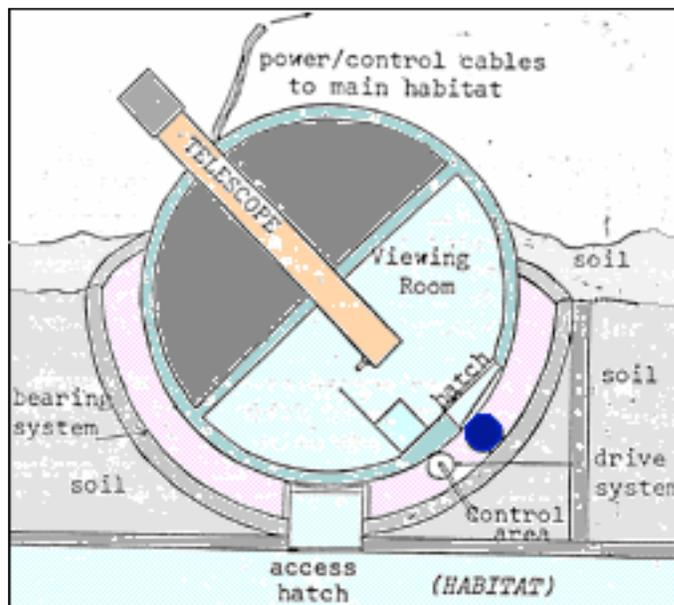
Submitted by Milwaukee School of Engineering (MSOE) student and MLRS member **Ron August** of Hubertus, Wisconsin, this concept involves a moving, spherical shaped viewing room, with the telescope an integral part of it, that is completely pressurized, heated, and accessible from the habitat below. Entrance to the room is by way of an airtight hatch system.
