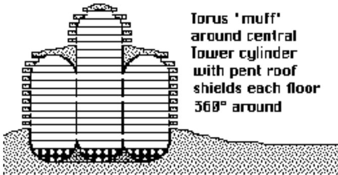
The inner and outer walls of the stretched torus would have to be constrained to shape by floor-incorporated cables under tension.
