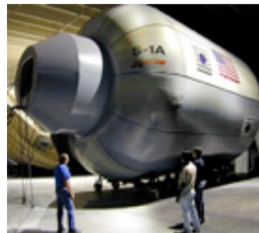
Inexpensive, @ \$100 million delivered to orbit, the **B330** can be configured into 2 and a half floors. Outfitting apparatus must be designed to fit through its airlock b/4 unfolding. This could be done in Earth orbit.
