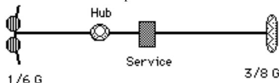
The Service Complex can be positioned anywhere along the axis, to either side of the hub as needed to balance the Lunar and Martian Wings.
