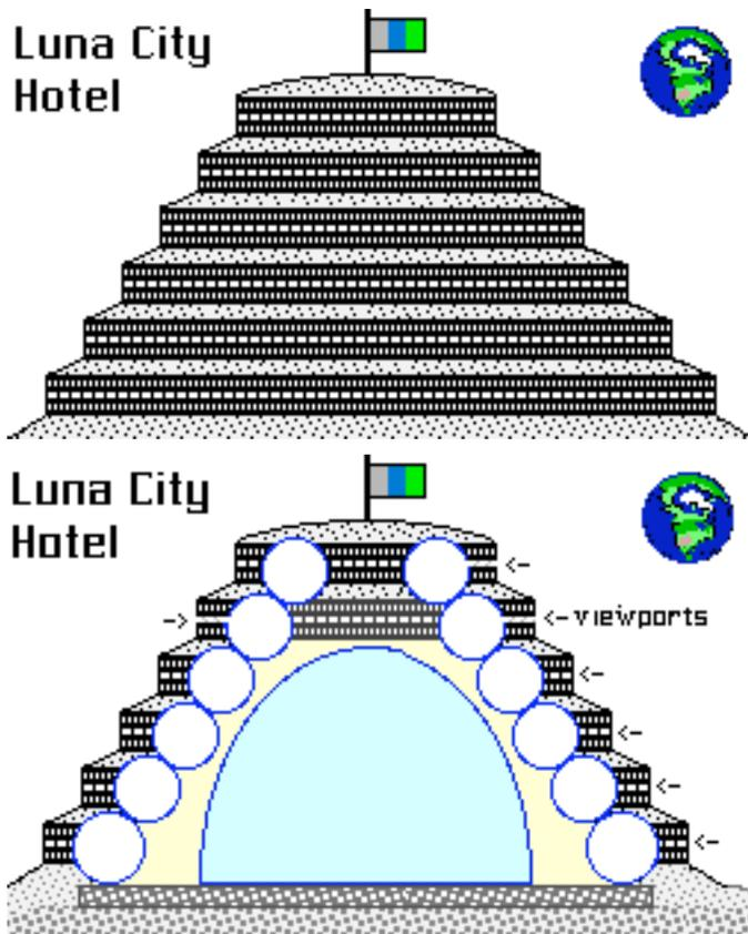
Each tier or “story” consists of a torus of successively smaller diameter, each resting in contact on the one below. The empty space below is put to good use with an atrium garden.
