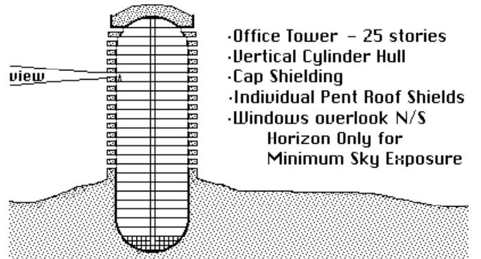
What appears to be tiers of balconies, in this sketch, are really continuous cantilevered coffer dams filled with loose regolith soil shielding. Building occupants are restricted to the interior of the fixed pressure-holding windows to the inside of these “pent roofs”.
