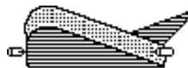
Hybrid Mars dirigible aircraft Thick Delta Wing holds hydrogen gas, is shaped for speed. M. Clapp
