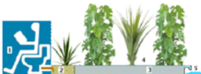
KEY: 1 side- or wall-flush toilet; 2 blackwater tank with microbes to break down solids & destroy pathogens; 3 inert filter with irrigated soil; 4 plants rooted in wet soil mixture; 5 effluent water is 95% pretreated, ready to water plants in the greenhouse and elsewhere. - illustration by the author.
