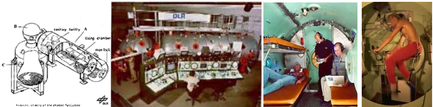
Figure 1. (a, b, c) Titan Hyperbaric Chamber used for the EXEMSI campaign, (d) a test subject exercising on a bike ergometer (Source: DLR)
