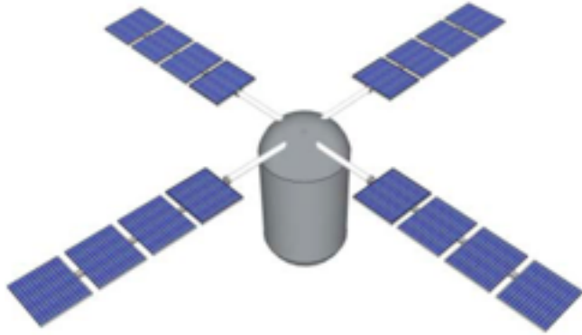
Figure 7: Solar panels on the Farm Module. The above picture shows a possible layout for the utilization of solar panels at the far end of the "Farm" module to augment power provided from the ISS.
