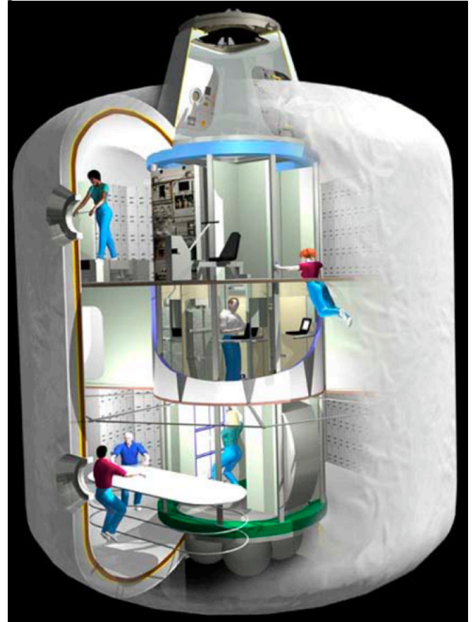
Figure 4: NASA's Proposed TransHab Module. Above is a conceptual drawing of the compartmentalized inflatable TransHab module that would have replaced current crew quarters onboard the International Space Station. http://www.life.com/image/50703432
