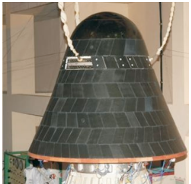
Test recovery capsule for ISRO Manned Spacecraft
