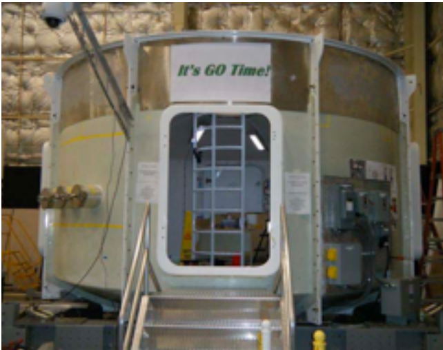
NASA's "X-Hab" lower floor to which is to be mated an "inflatable loft" the design of which is the subject of a competition: http://www.spacegrant.org/xhab/2011 Read "Exploring the Many Possibilities of Hybrid Rigid-Inflatable Structures" pages XX-XX, below
