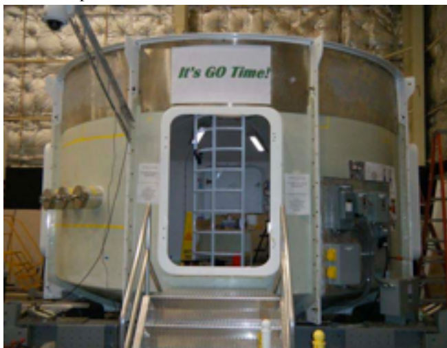
NASA X-HAB inflatable loft competition: Loft to be attached to top ring of hab structure above http://www.spacegrant.org/xhab/2011
